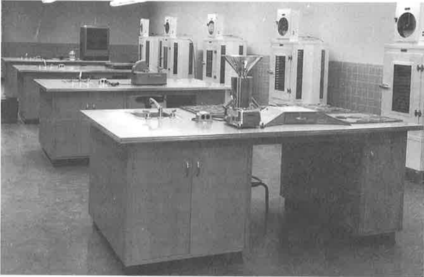
Figure 5. View of the seed germination laboratory. Each center island had a small sink and provided space for two analysts with a vacuum line for each to plant seeds. Two walk-in germinators (not shown) were available as well as small germinators located along the back wall.
